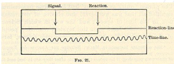
One type is that of the revolving drum covered with smoked paper, on which one electric pen traces a line which the signal breaks and the 'reaction' draws again; whilst another electric pen (connected with a pendulum or a rod of metal vibrating at a known rate) traces alongside of the former line a 'time-line' of which each undulation or link stands for a certain fraction of a second, and against which the
